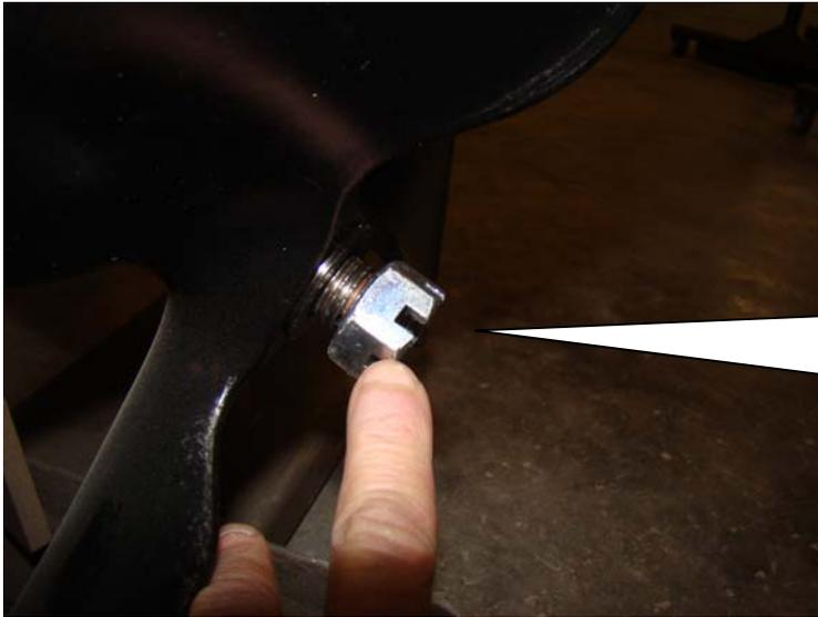
**To install the prop first coat the spline and thread with Locktite marine grade anti seize or equivalent and secure nut.**
