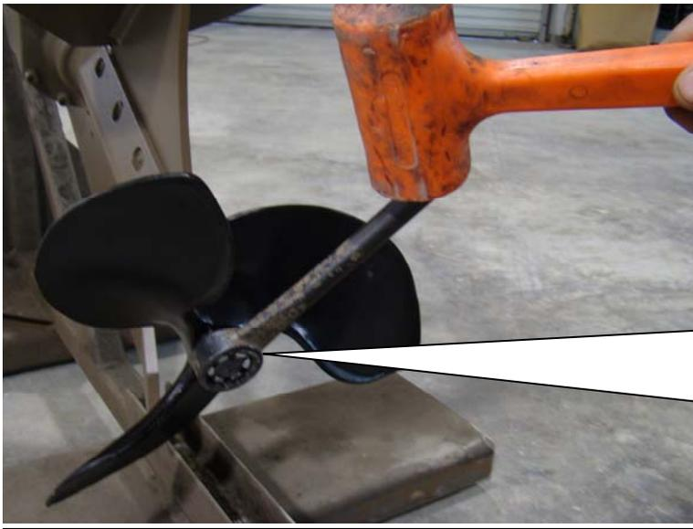
**Using your 1-1/8" wrench tighten the prop. Next lightly tap the wrench to further tighten the nut to align the prop shaft hole with one of the slots in the nut. Install cotter pin.**
