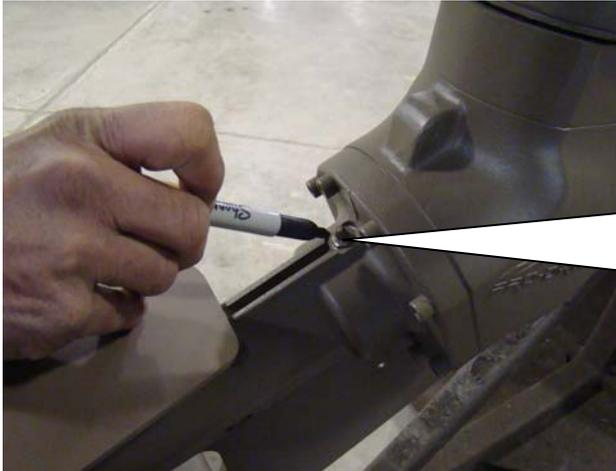
**REMOVE ANY GRASS OR FOREIGN DEBRIS FROM THE PROP SHAFT BETWEEN THE PROP AND LOWER UNIT HOUSING. PUMP GREASE INTO THIS GREASE FITTING EVERY 15 to 20 HOURS**
