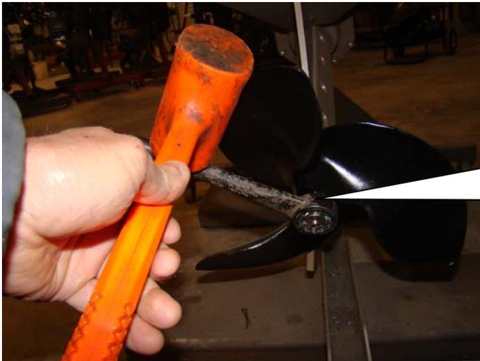
**Using a 1-1/8" wrench and a light hammer blow unscrew the nut counter clockwise. Prop can now be slide off spline.**
