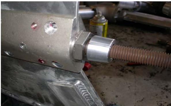
**INSTALL THE TAPERED BUSHING AS SHOWN, MAKING SURE THAT IT IS FULLY FORWARD AND BOTTOMING OUT AT THE THREADS END. COAT THE OUTSIDE DIAMETER OF THE BUSHING AS IN THE ABOVE STEP.**
