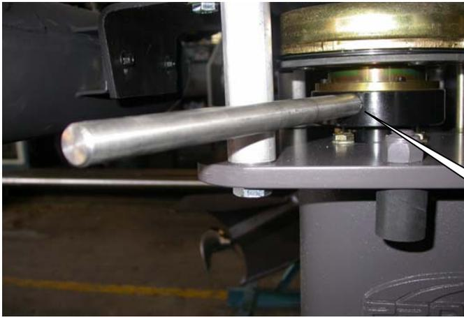
**REMOVE THE CLUTCH COVER WRAP AND LOCATE THE HOLE STOP AS SHOWN ON LEFT. INSERT 1/2" BOLT OR PROP PIN INTO THE HOLE STOP. (THE PIN WILL PUSH UP AGAINST THE PLATE POST AS BACK UP WHILE UNSCREWING THE PROP.) \*NOTE: THE PROP UNSCREWS TO THE LEFT.**
