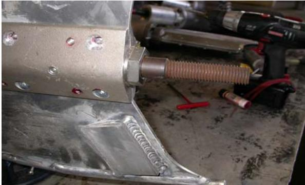
**USING LOCKTITE MARINE GRADE ANT-SEIZE OR NEVER SEIZE COAT THE ENTIRE SHAFT.**
