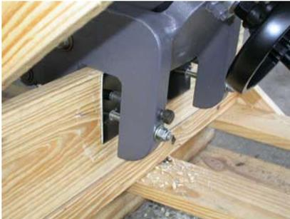
THIS PICTURE OF A UNIT CRATED FOR SHIPMENT SHOWS THE ALL THREAD INSTALLED THROUGH THE TRANSOM SAVER PLATE.
