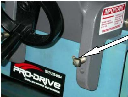
AFTER INSTALLING YOUR MOTOR ON THE BOAT TRANSOM USING THE ALUMINUM SAVER PLATE SUPPLIED WITH THE UNIT, TORQUE THE TRANSOM BOLTS TO 15 FT. LBS. OF TORQUE.
