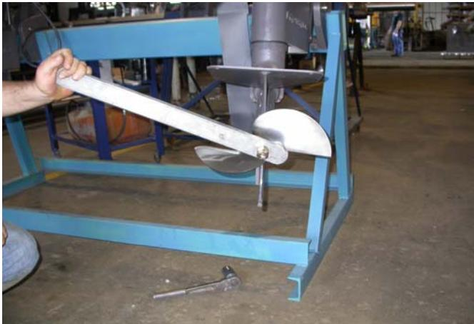
**REMOVE PROP NUT USING A 1-1/16" WRENCH OR DEEP WALL SOCKET. NEXT, INSTALL THE PROP WRENCH AS SHOWN. REPLACE NUT TO ENSURE THAT THE PROP WRENCH WILL NOT SLIP OFF WHEN REMOVING PROP. TURN THE WRENCH COUNTER CLOCKWISE UNTIL THE PROP IS REMOVED.**
